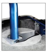
Body-mounted inner brackets strengthen the tire carrier for a solid installation.
