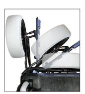
The tire carrier and tailgate swing out as a single unit.
